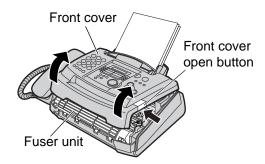
When the recording paper has jammed near the drum and toner unit:
